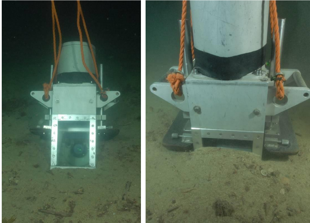
Figure 2.1. Diver operated Sediment Profile Imaging camera. The left-hand image gives a view of the camera at the sediment surface. The right-hand image shows the SPI camera when inserted into the sediment.
