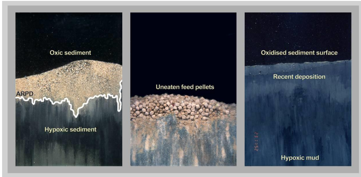
Figure 2.2. Typical sediment profile images with examples of features.
